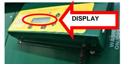
Upon the temperature of Boiler Tank dropping down to the pre-set value, LCD shows READY status. Residue Drain Valve located at the bottom of the Boiler Tank may be opened to drain all oily residues into Residue Drawer as shown in the photo.
