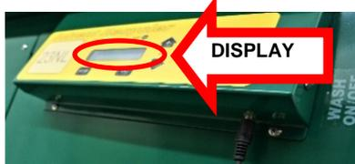
The liquid crystal display (LCD) located in Key Panel (shown on the left) displays variety of messages of up to 32 characters (16 characters in two lines). These messages are vital communication to operator as well as to service technician and include process status messages, relevant temperature data, user set-up messages, Manual Mode messages, Test Mode messages, Factory Set-up messages, error and caution messages, Data logging messages, etc.
