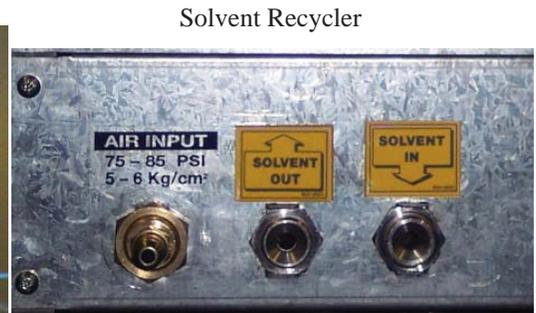
Attach Moisture Filter (optional) to Air Input and the Tee to the Filter (if used) and the Blue Airline to Tee and Gun Cleaner. The Air Supply fitting is also not supplied.
